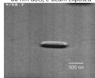
Fig.8c: 0.8 µm wide niobium dot after resist remove
